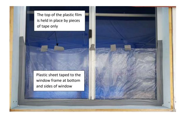
The following photographs show the efficiency of the plastic film in containing the water during a simulated cyclone wind gust. Rain was simulated by spraying water on the window. With the plastic film set-up, the water is contained and returns outdoors through the window weep holes after the wind gust instead of causing water damage to the inside of the building.
