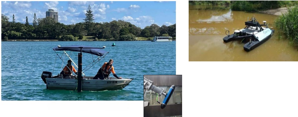
Figure 5 Staffed bathymetric boat (left) and remote controlled bathymetric vessel (right) used for data collection (courtesy of Woolpert Australia Pty Ltd).
