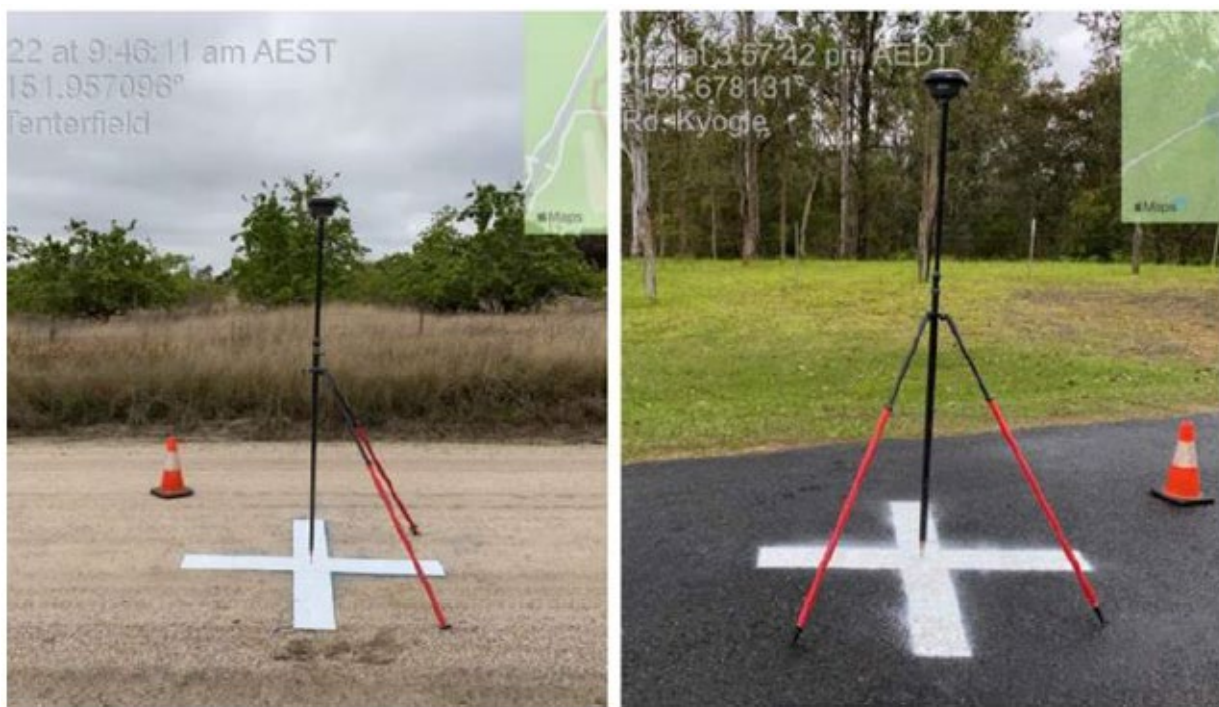
Figure 3 Example of ground control points installations –in Tenterfield (left) and Kyogle (right) (courtesy Fugro).
